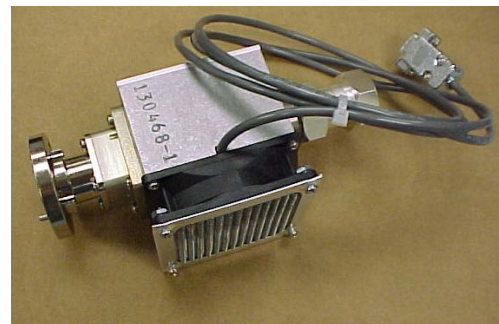
Illustration 2-10 Directional Coupler port and directional coupler
