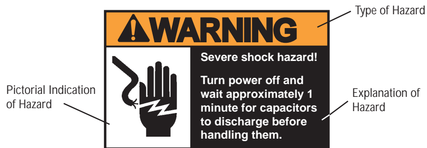
Illustration 1–3 Sample Hazard Alert
