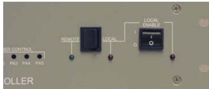
Illustration 3-5 Remote/Local and Local Enable switches with indicators
